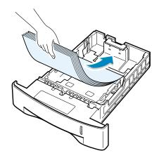
You can load previously printed paper. The printed side should be facing up with an uncurled edge at the top side. If you experience problems with paper feed, turn the paper around.
